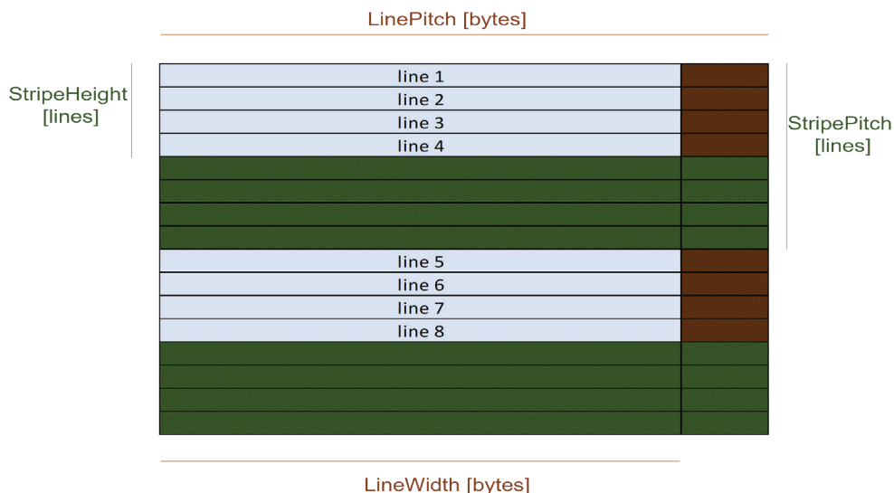
Figure 1: Frame Components of Bank A Sub-frame for S641
