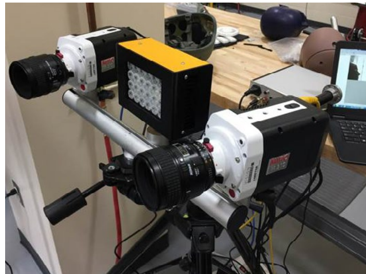
Figure 4: Camera set-up of Miro 310s for experiment
