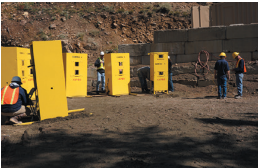
Students setup Phantom cameras inside specially built cabinets.
