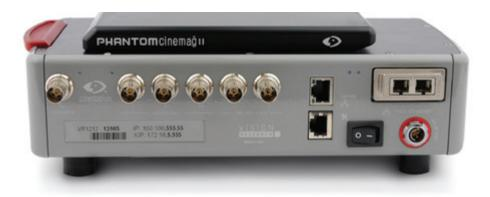
Phantom CineMag II installed on a Phantom CineStation-X2SR
