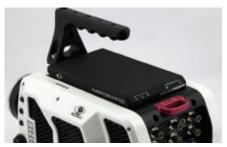
CineMag II installed on a Phantom v1210 camera
