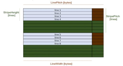
Figure 1: Frame Components of Bank A Sub-frame
