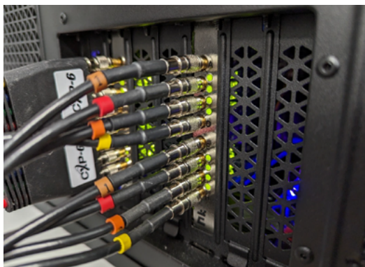
Figure 4 – CXP-6 cables plugged into the EureSYS Coaxlink Octo.
