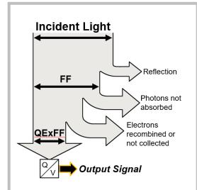
**Quantum Efficiency**<sub>( $\lambda$ )</sub> (QE) – ratio defined by the number of electrons generated per photon of wavelength  $\lambda$
