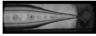
Figure 1 shows an example of a microfluidics study, in which two different fluids were mixed and the resulting tiny droplets were studied. The image is from a sequence captured at 10,000 fps with a 20 microsecond exposure, using a Phantom Miro LC310 monochrome high-speed camera and Leica microscope.
